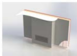
Fig 2. Uses an air outlet opening at the top of the enclosure that is built-in at the top, centered above the appliance. This allows the heat to escape into the same room as the fireplace.
